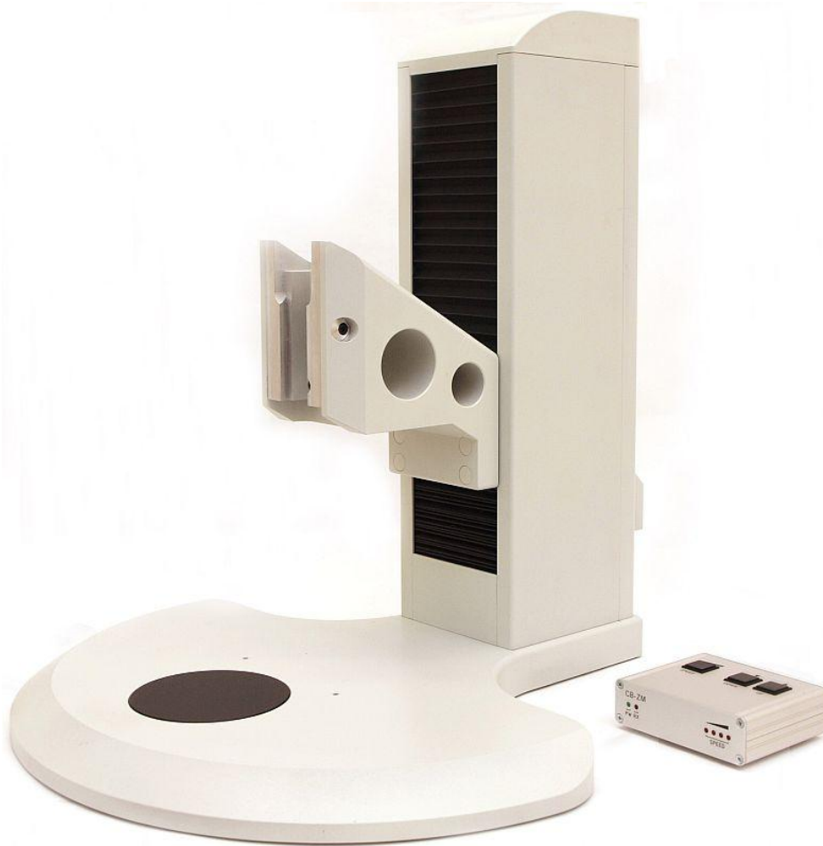
PRO-MLS stand with PRO-ZBAD adapter and CB-ZM control unit
