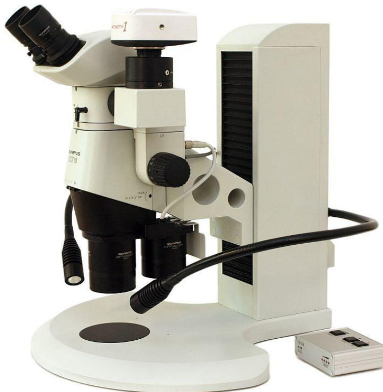
Motorization of OLYMPUS® SZX16 stereomicroscope
